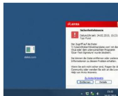
**Eicar test file for virus scanners:** The Eicar Institute became known with this harmless test file.
